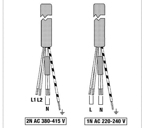
2. For single-phase connection, connect the wires as identified below:
