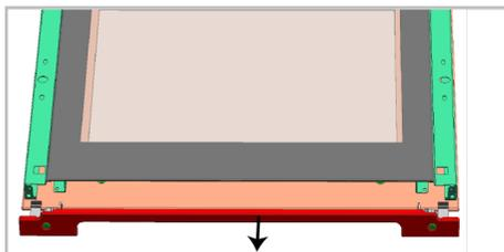
2. As illustrated in the figures above, press on the tabs (1) and pull the profile (3) towards yourself simultaneously to remove the profile attached to the upper side of the front door.
