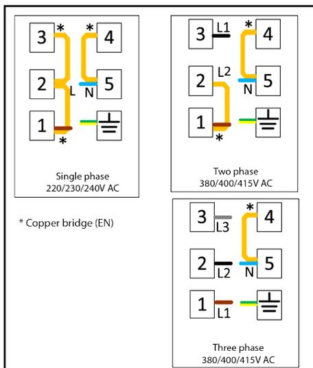
If your supply cord type is 3-conductor type, for 1-phase connection:
