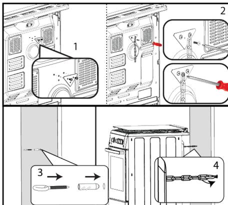
**i** Stability chain to be as short as practicable to avoid oven tilting forward and diagonal to avoid oven side tilting. Stability chain is designed for cookers without a bracket engagement slot.
