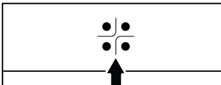
Hot zone warning indicator shows the position of the turned on hob, and it remains lit after it is turned off. A flickering light on the hot zone warning indicator is not a malfunction.
