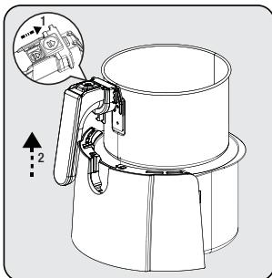
Press the basket release button (4) and raise and pull up the handle (5) upwards and thus take the removable cooking basket (7) out.
