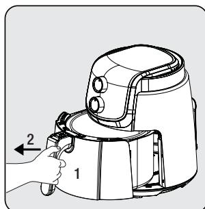
Grab firmly the handle of the removable cooking basket (7) to open up the basket drawer (6); then, take the drawer out of the appliance and position on a flat and clean surface.
