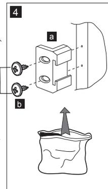
**Note:** Installation step for 3, screws for connecting top plastic part should not be screwed very hard, because of moving the plastic part easily left or right side.
