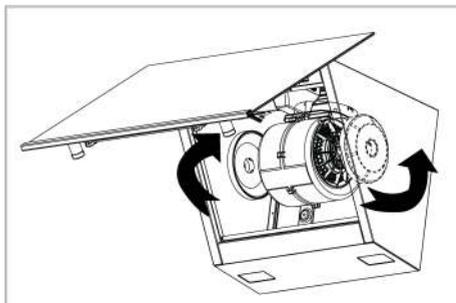
3. Place the lug slots of your new carbon filters into the lugs on the motor holder and turn them clockwise to snap them into place.
