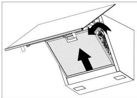
3. Reinstall the aluminium filter in its slot after flushing by following the above steps in reverse.
