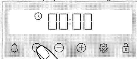
**i** After setting the operation function and temperature, you can set the cooking time for 30 minutes by touching the ⊕ key directly for quick setting of the cooking time and change the time with the ⊕/⊖ keys.
