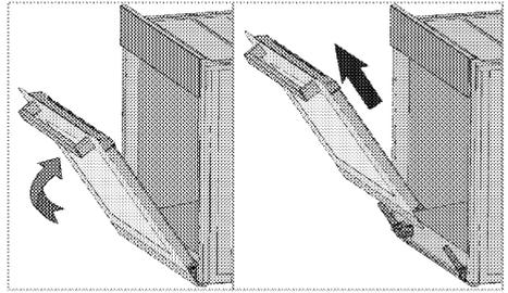
4. Pull the removed door upwards to release it from the right and left hinges and remove it.
