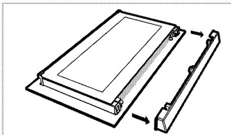
3. As shown in the figure, gently lift the innermost glass towards 'A' and then, remove it by pulling towards 'B'.
