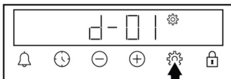
2. Set the desired brightness with the (+)/(-) keys. (**d-01-d-02-d-03**)
