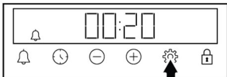
⇒ After setting the alarm time, the symbol remains lit and the alarm time starts to countdown on the display. If the alarm time and baking time are set at the same time, the shorter time is shown on the display.
