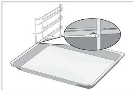
**Proper placement of the wire grill and tray on the telescopic rails-On models with wire shelves and telescopic models**
