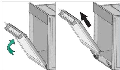
8. Pull the removed door upwards to release it from the right and left hinges and remove it.
